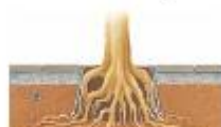
The established tree roots spread below the barrier where secondary thickening does not harm paving. Deeper root growth also improves tree stability and drought resistance.
