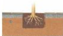
Standard tree planting for street tree in unprotected tree pit.
