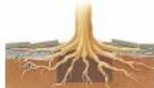
As the tree grows the roots undergo secondary thickening which begins to lift paving and cause extensive damage. Cutting roots to repair paving or excavating the service pipe will seriously destabilise the tree, probably leading to its death and removal.
