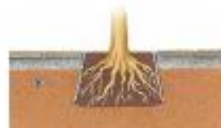
As the tree establishes, the roots spread out and are guided downwards and outwards by the root director walls and integral ribs.
